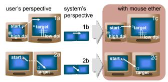
Figure 1: (a) When trying to move the mouse pointer straight to a target on the other screen of a multimon setup the pointer gets warped, because (b) the system is oblivious of resolution differences and gaps. (c) Mouse ether eliminates warping.
