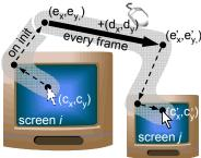
Figure 2: Mouse ether processing a mouse move
