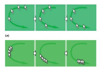
1 High-density cursor versus mouse trail. Unlike the (a) similar mouse trail technology, the (b) high-density cursor uses temporal supersampling to bridge gaps in the cursor's position without lag.
