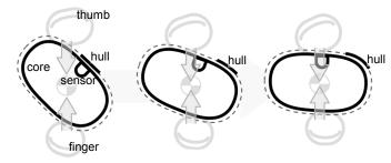
**figure 2:** The mechanics of soap: As the user applies pressure using thumb and finger, the core rotates to evade the pressure. At the same time, friction between finger and hull holds the hull in place, resulting in relative motion between hull and core.
