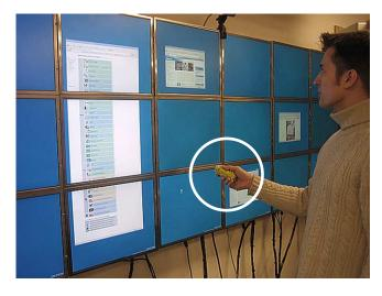
figure 5: Using soap to interact with an 18-panel wall display.
