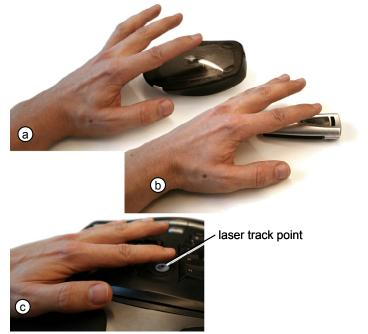
Figure 7: Three prototypes we used to simulate a motion scanner device: (a) Optical mouse on its back, (b) Xybernaut Poma, and (c) laser track point.
