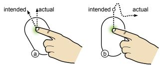
Figure 9: Errors resulted from (a) inadvertent rotation of the device and (b) incomplete lift-off.
